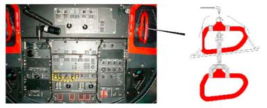
Actuating one general CUT-OUT handles shuts off both engines and cuts off all the electrical supplies except the engine fire extinguishing systems and some necessary items (triple NR indicator...).
