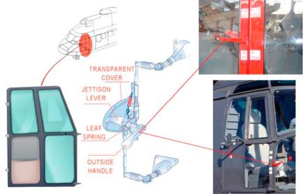
Doors can be jettisoned by actuating the jettison lever, secured by a leaf spring and protected by a breakable transparent cover. It causes the door to fall away. It can be operated from the outside by the outside handle.
