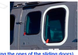
Fixed windows (including the ones of the sliding doors) are jettisonable from inside or outside by pushing out strongly after removing the seal-retaining strip.
