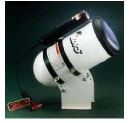
In most cases, the parachute deploys up and aft and the entire assembly is located close to the aircraft center of gravity-around where the wing and fuselage meet. If this rocket were to deploy from an accident aircraft on the ground and someone at the accident site was in the way, the result would likely be a fatality. Most aircraft will have a triangular warning label that indicates where the rocket leaves the aircraft. If you see that triangular warning label, you should avoid that area.
