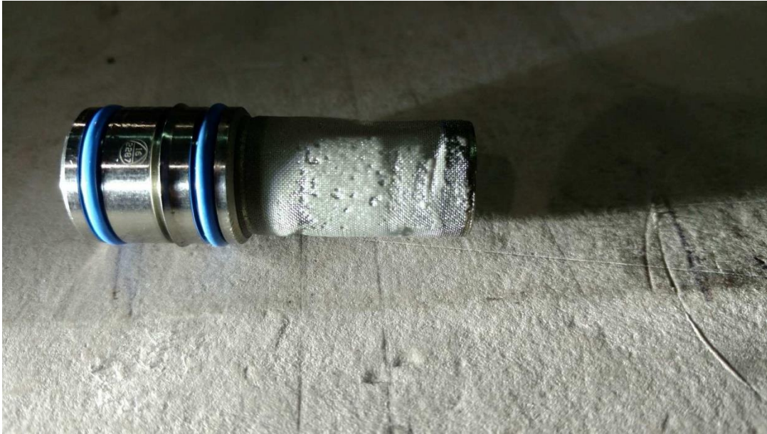
Figure 2: DEF crystallization on aircraft fuel filter.
