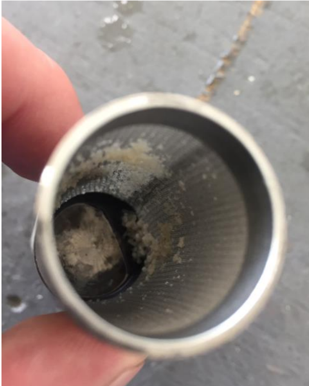
Figure 1: DEF crystallization on aircraft fuel screen.
