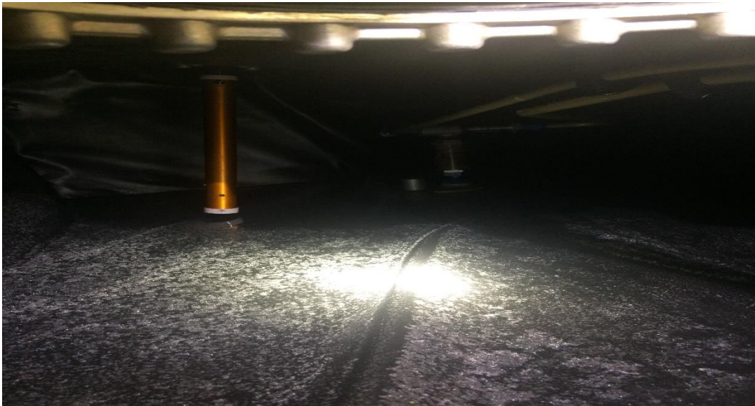
Figure 3: DEF crystallization in aircraft fuel tank.
